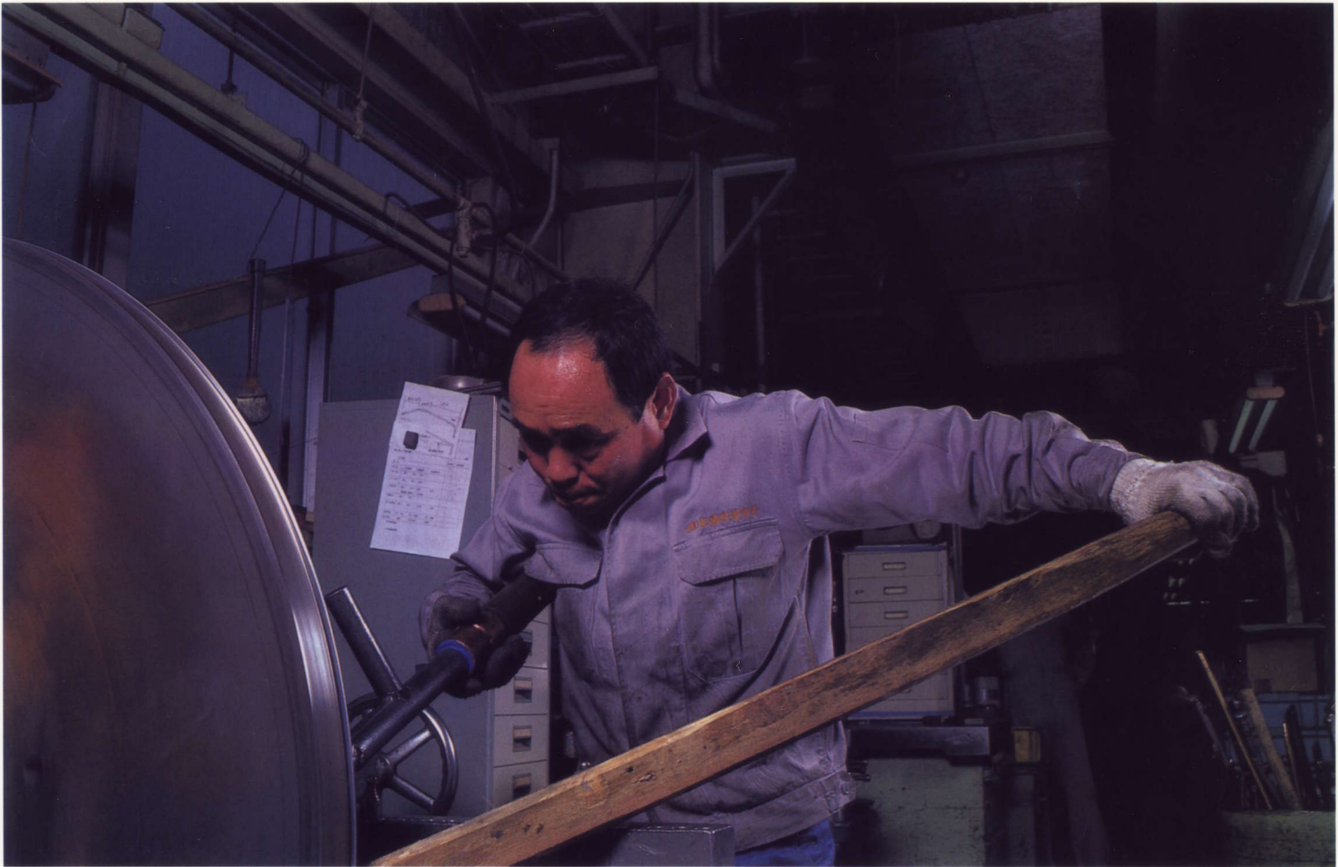
A spatula tool is used to apply pressure to the rotating metal disc to force it into a cylindrical shape. It takes about 10 years to learn exactly how much pressure to apply.
