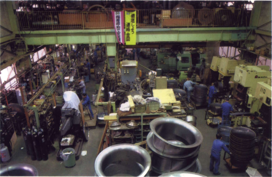
Kitajima Shibori Seisakusyo's factory. A host of products, ranging from a parabolic disc over 2m in diameter to a product not more than 3mm in diameter, is made by applying spatulas to rotating discs of metal.
